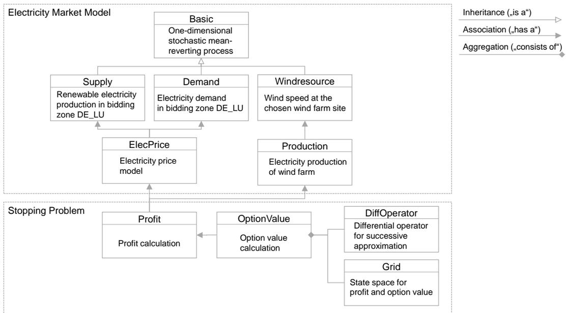
Figure B.5: Proposed class diagram for implementation
